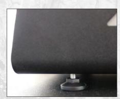
The adjustment of the support foot allows the machine to adapt to any surface.
