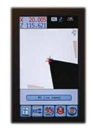
Automatic cutting edge measure. After having found the central position by means of focus bars, on the axes counters the measurement is shown without additional operations
