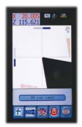
Tool profile collimation on fix reticule with X and Z axes analog comparators: axes control bars for the exact central position of the measure
