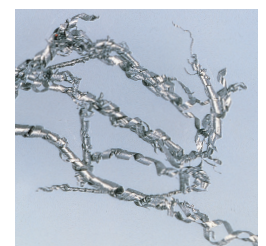
Swarf by reaming blade
