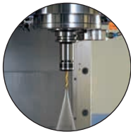
High Pressure Flange Through (MAX. 7MPa)
