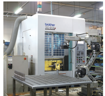
CNC table on TC-31A (pallet changer)+ work change by robot
