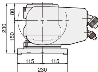
■ The Area of Noninterference in Tilting Position.
