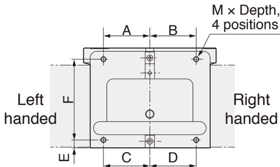
● Please refer to the above dimensions for direct mounting with the bolts from base plane side.
