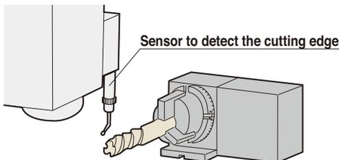
Sensor to detect the cutting edge
