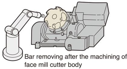
Bar removing after the machining of face mill cutter body
