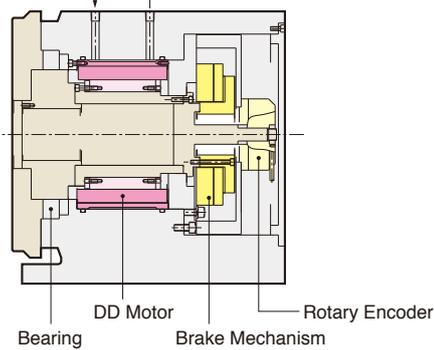
There is no mechanical reduction mechanism such as worm system in a rotary table with DD motor. DD (Direct Drive) motor is built in the the rotary table to drive directly. High rotation speed and high acceleration/deceleration can be done. However, the driving torque of the rotary table is not strong due to no mechanical reduction mechanism. Therefore, the suitable application of the rotary table with DD motor must be selected.
