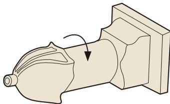
Simultaneous 3 axes control of X, Z & A axis instead of turning.
