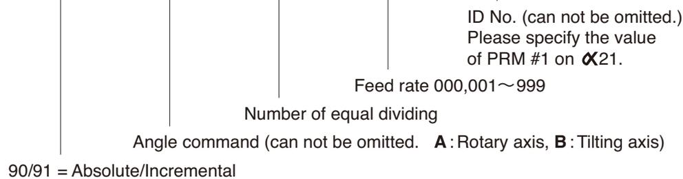
M21(start) will be executed as required times after execution of macro program for direct angle command.
