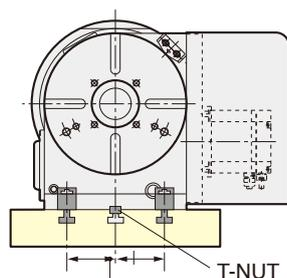
CLAMPING DEVICE is designed for T-slot pitches of 100mm or 125mm on the machine bed table. Please contact with us for the other pitches.
