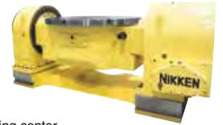
5AX-1200A is also available. The face plate is located above the center of the tilting axis.
