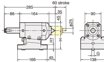
The center height can be adjusted within 0.35mm.
