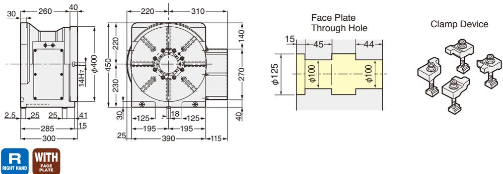
**Specifications** The external dimension and the specification will be varied according to the DD motor. Please contact us.
