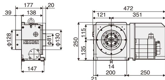
External dimensions depend on the type of the servo motor. Indicated dimensions are in case of FANUC. Please contact us for CAD files (2D:DXF, 3D:PARASOLID).
