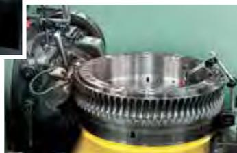
Hobbing of the gears with large module
