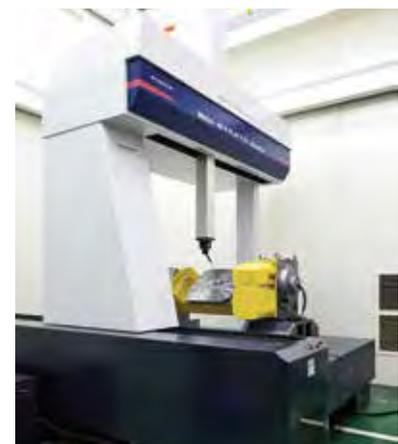
Accuracy measurement with large 3 Dimensional Measuring Machine
