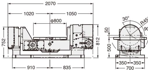
1. Moving angle of the tilting axis
