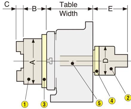
When power chuck or rotary cylinder is installed on 5AX-table, the 5AX-table must be High Column type.
