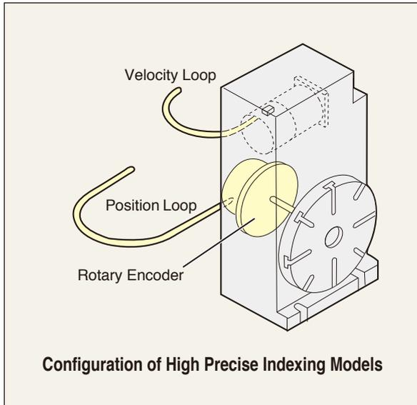
Full closed loop control becomes possible by mounting a rotary encoder at the back of rotary table. And high precise indexing becomes possible by detecting the rotary angle of the table directly.
