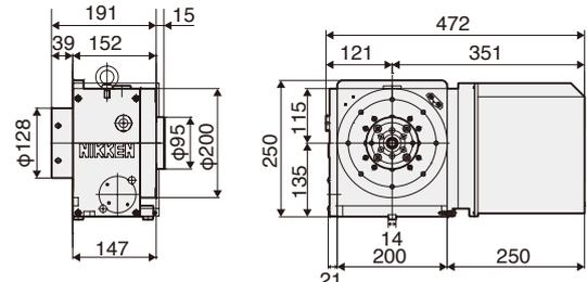
External dimensions depend on the type of the servo motor. Indicated dimensions are in case of FANUC. Please contact us for CAD files (2D:DXF, 3D:PARASOLID).
