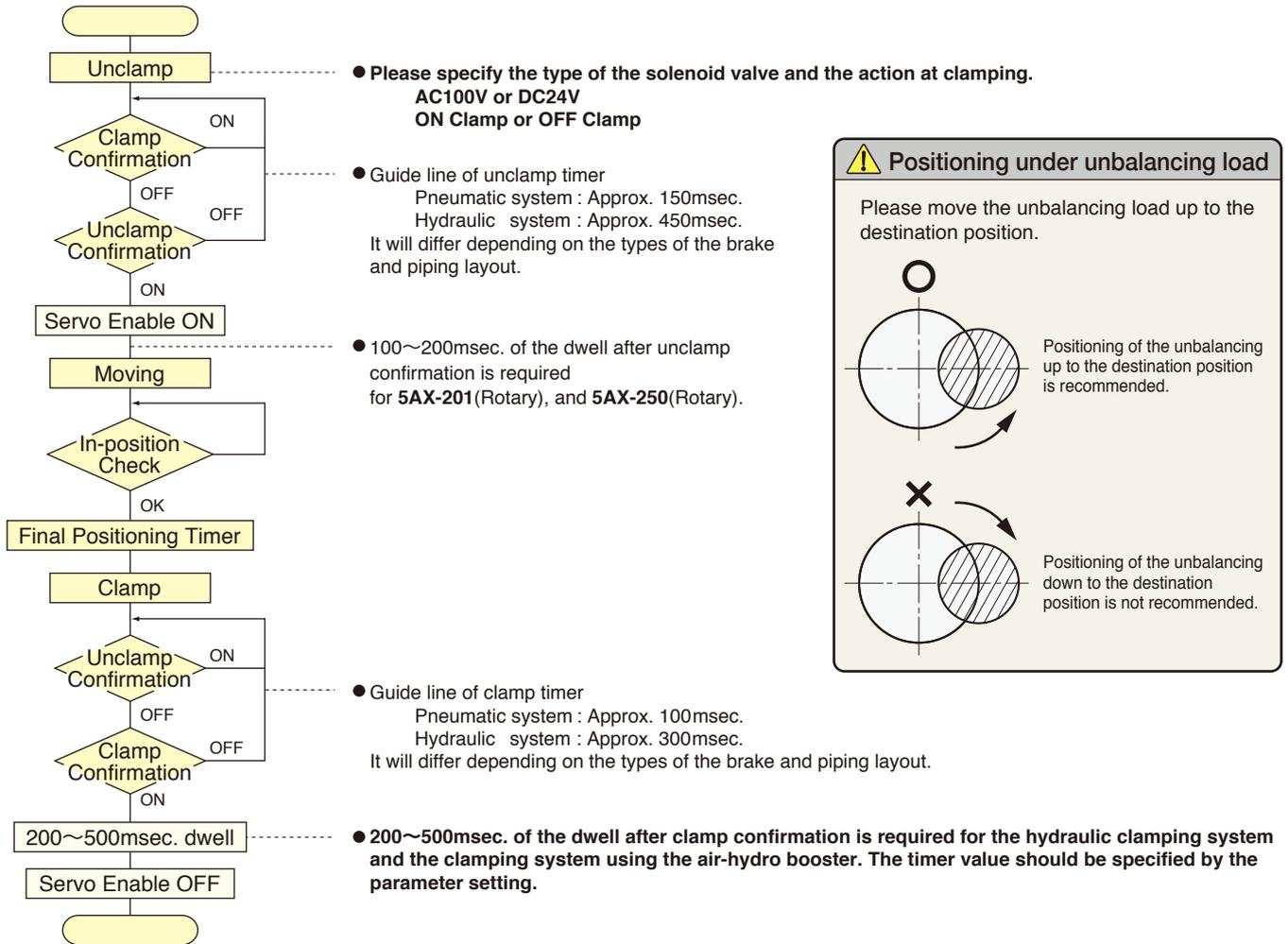
**⚠ Positioning under unbalancing load**
