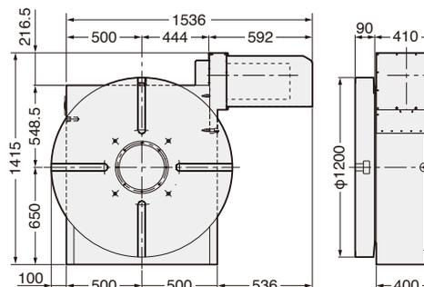
★ Ultra precision of  $\pm 3\text{sec}$ . is available as an option. There is no through hole on the rotary table due to the rotary encoder for ultra precision option.
