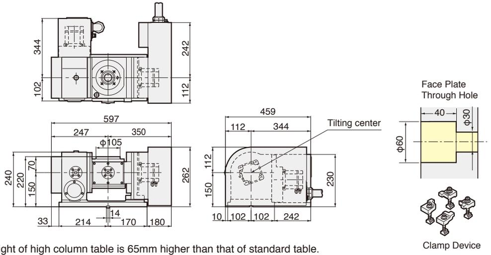
Center height of high column table is 65mm higher than that of standard table.
