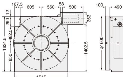
★ Ultra precision of  $\pm 3\text{sec}$ . is available as an option. There is no through hole on the rotary table due to the rotary encoder for ultra precision option.
