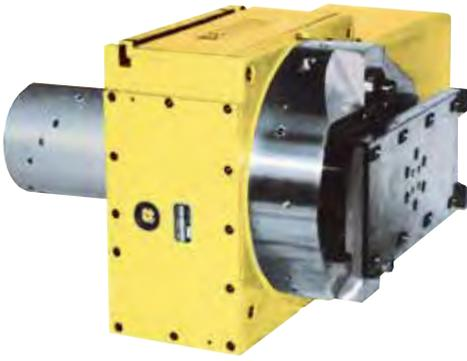
Rotary Joint is a rotating connector to supply air, hydraulic pressure or coolant liquid from outside to a fixture on a CNC rotary table. If liquid is supplied with ordinary hoses, twisting will happen on them by rotation of the table. However, rotary joints can solve this problem as it rotates in accordance with the table.
