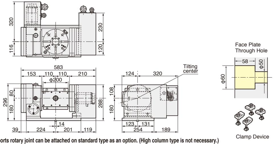
Built-in type 4 ports rotary joint can be attached on standard type as an option. (High column type is not necessary.)
