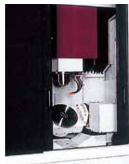
Utilization for 4th and 5th axis rotary table of the M/C for die molding
