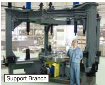
CNC1800 & Support Branch Indexing/ clamping of the turbine disk
