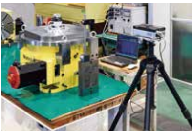
Indexing Accuracy Measurement by Laser
