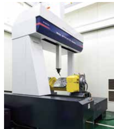
Accuracy measurement with large 3 Dimensional Measuring Machine
