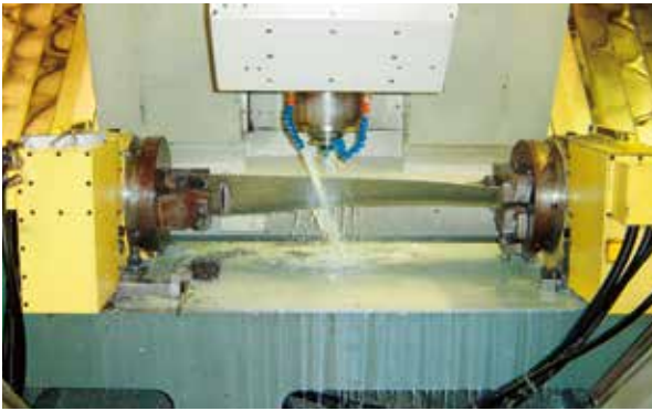
Synchronous Rotation by CNC401 X 2units
